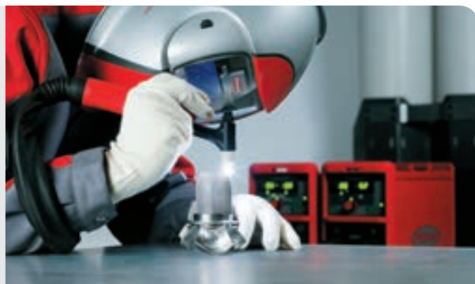
/ Manual microplasma welding for sheet thicknesses from 0.1 mm (0.004 in.) upward.
